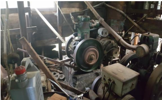
This old LISTER engine still runs & powers all the machines in the Boat building shed, using numerous flat belts that once in operation, whistle around at a rate ok knots,
